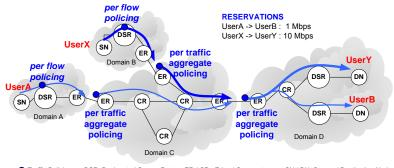
• Traffic Policing DSR: Designated Source Router ER / CR : Edge / Core router SN / DN: Source / Destination Node Figure 7. Traffic control in DiffServ network (inter-domain scenario)
