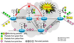
Figure 11. Generating alarms after a traffic reroute.
