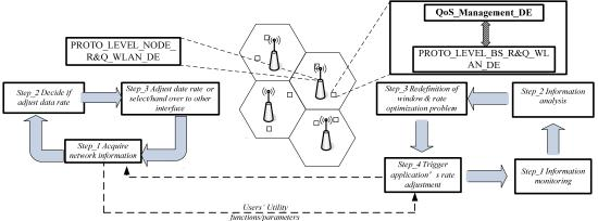
Figure 21. WLAN QoS related decision elements (DEs) and control loops in GANA
