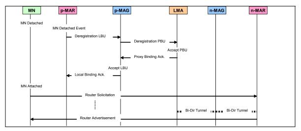
Figure 39. Inter MAG Handover – Signalling Sequence
