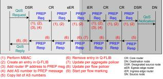
Figure 9. End-to-end Signaling.
