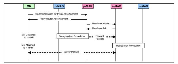
Figure 40. Fast Handover in HPMIPv6 Domain
