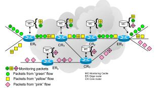
Figure 10. Handling monitoring packets by ingress and internal routers in a domain.
