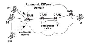
Figure 2. The simulation topology.
