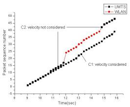
Figure 49. Impact on packet lost rate of velocity
