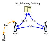
Figure 25. LTE Network Architecture
