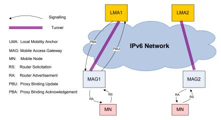
Figure 34. Proxy Mobile IPv6 Domain
