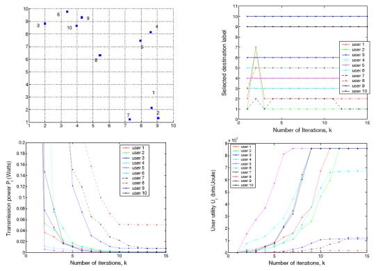
Figure 59. a) Network topology for 10 nodes; b) Users' destinations selection; c) Users utilities; d) User's transmission powers.
