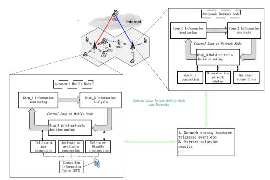
Figure 44. Connection Management Mechanism with Control Loops of GANA
