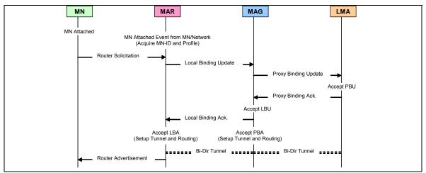
Figure 37. MN Attach – Signalling Sequence
