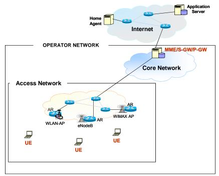
Figure 26. Heterogeneous Network Scenario
