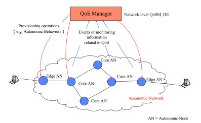
**Figure 1. Wired Network Architecture**
