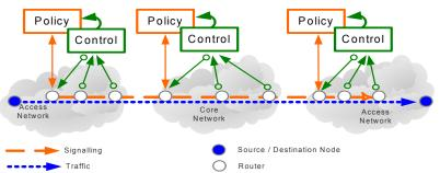
Figure 8. Control mechanisms in routers for autonomic control of flows and traffic policies
