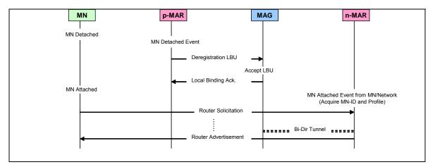
Figure 38. Intra MAG Handover – Signalling Sequence
