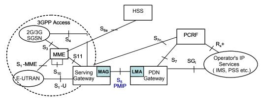
Figure 35. Architecture for 3GPP Accesses within EPS using PMIP-based S5
