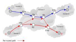
Figure 6. Congestion problems in Ra-Rb link due to rerouting of red flow.
