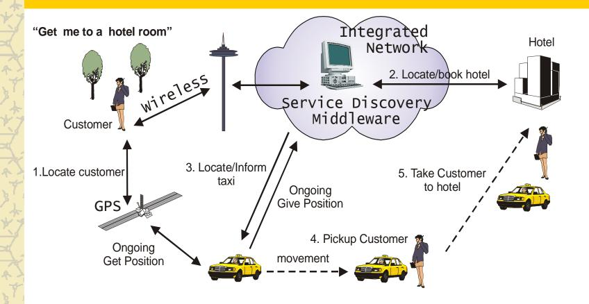
The criteria for service discovery can be the physical or network position (*Location-Based Services*), and can also exploit *User Profiling* technology
