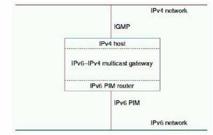
In IPv4 the gateway is a multicast host using IGMP
